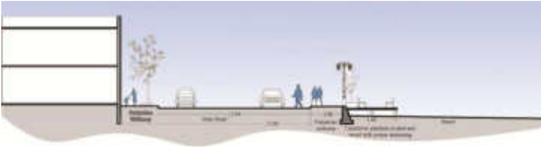
Section AA – Proposed decks in light weight material such as timber and steel with proper anchoring
