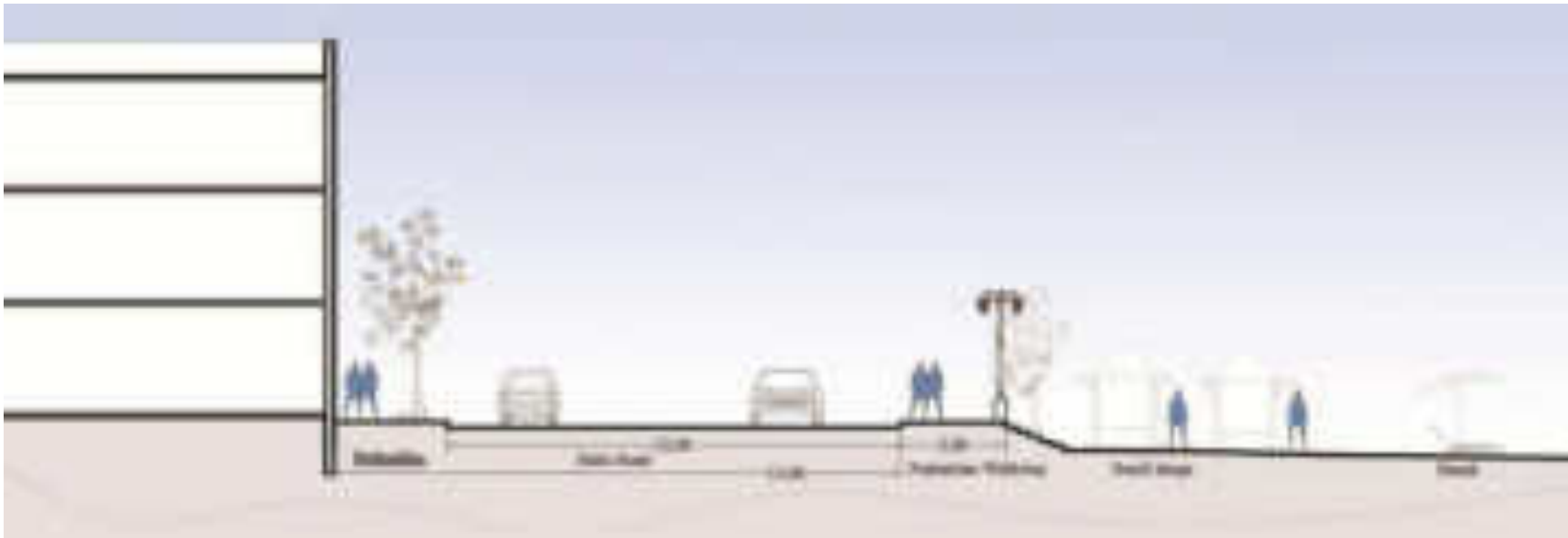
Section CC – The hawkers on the footpath are shifted on the beach, for proper pedestrian circulation (Small shops that are semi-permanent)
