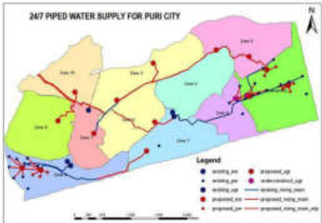
Map 8.9: Zoning and Detailed plan for water supply network as per DPR
